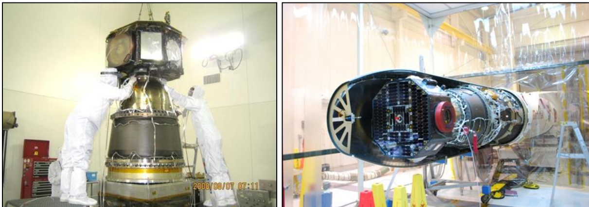
Figure 2-6: Three MkII MLBs (38.8, 31.6 and 15.0 inch diameter) are used on the IBEX Program.
