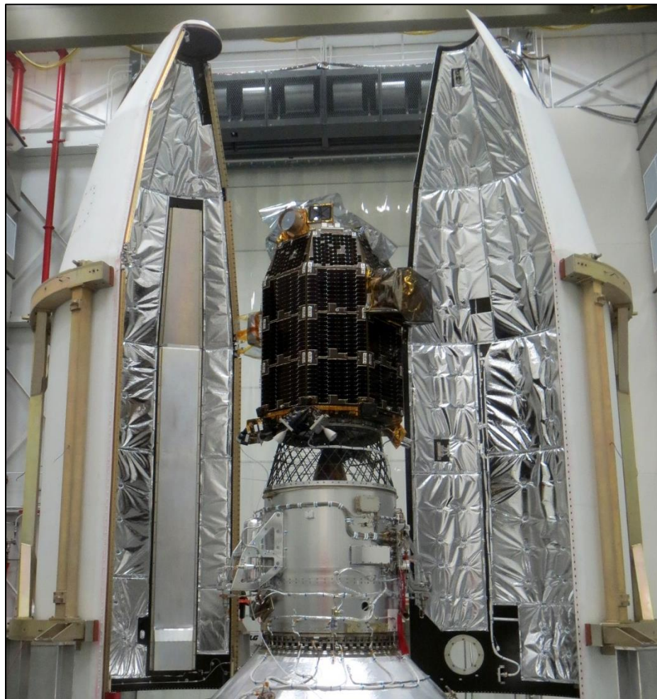
Figure 2-8: Two MLBs installed on a lunar payload prior to launch 1
