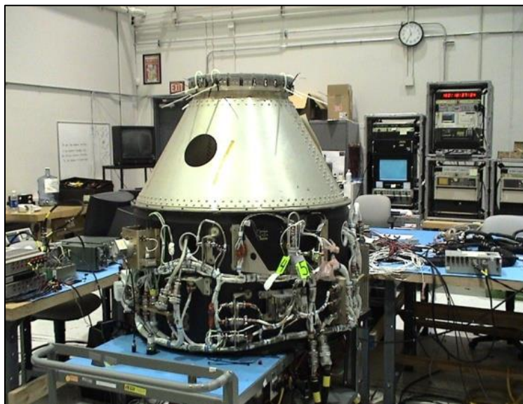
Figure 20-1: Electro-mechanical fit check and a separation test with an MLB
