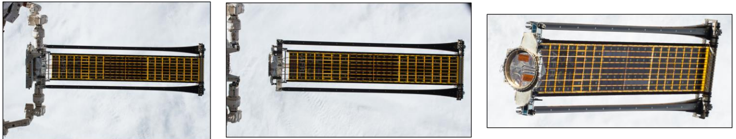
Figure 14-1: 23 inch MLB deploying ROSA from ISS
