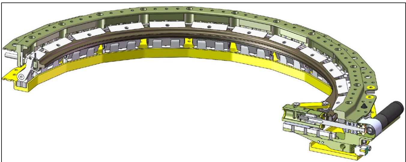
Figure 7-6: The Leaves disengaged during deployment, (section view)
