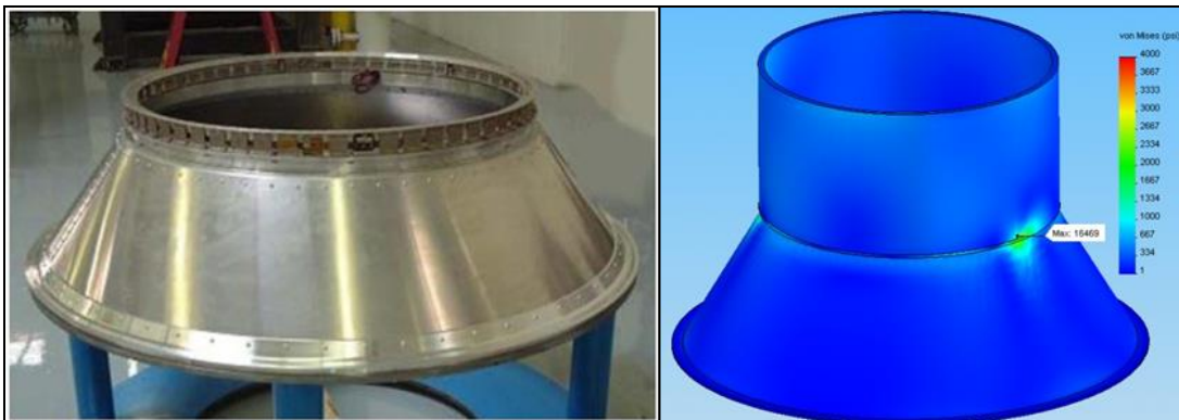
Figure 7-23: An MLB attached to a launch vehicle cone and CAD model showing resulting stress peaking that occurs when adjoining two warped surfaces
